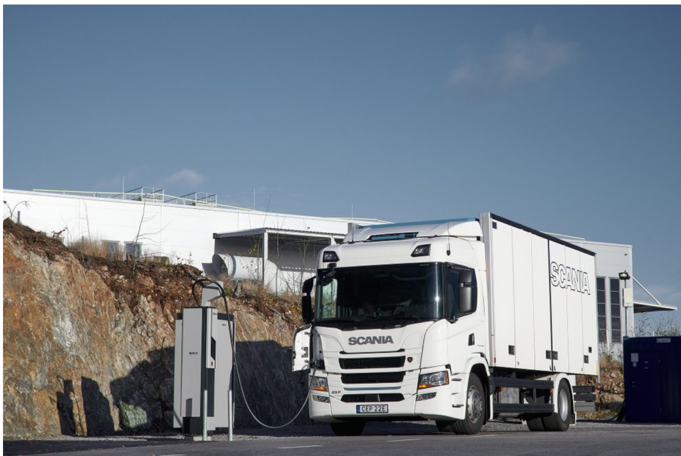
Scania 25 P BEV Charging station
